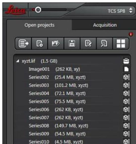
**Figure 3.2.** The Open Projects icon under the Acquire menu provides access to various drives and files available within the LAS X software.
