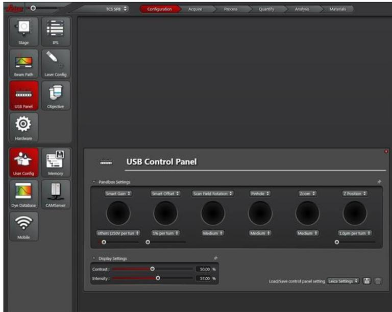
**Figure 2.7** LAS X Overview of the USB Control Panel Icon. Here the functions on the Leica Smart Control Panel can be adjusted. Each knob is assigned a parameter by selecting from the top drop down menu and the sensitivity of each turn is set with the bottom dropdown menu.
