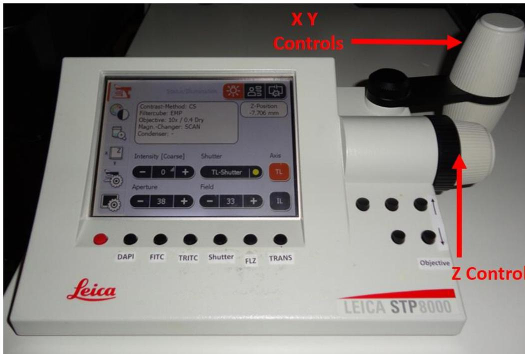
**Figure 1.9** Leica Smart Touch Panel overview. This panel provides access to various icons including the a) Microscope icon, b) Color Wheel icon, c) Objective icon, d) X, Y, and Z Stage icon, and e) two system setting icons. The arrows indicate knobs that allow the user to move the stage in the X and Y direction, as well as in the Z direction.
