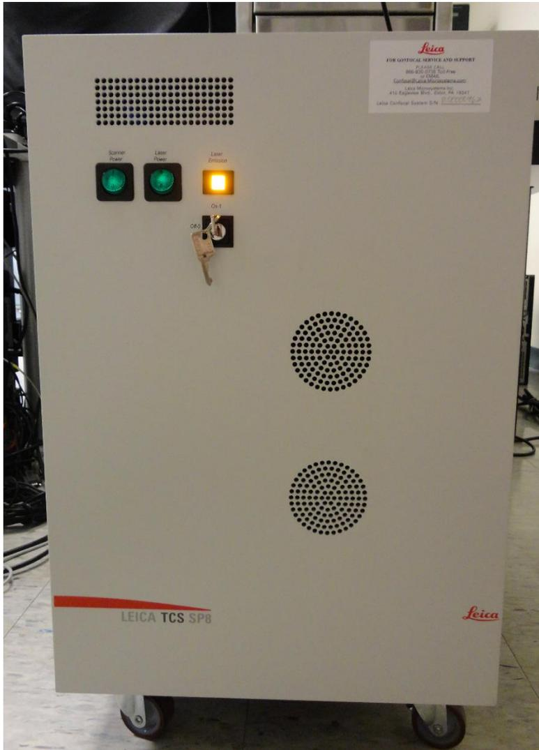
**Figure 1.3** Scanner and Laser power can be turned on here. The key should be switched to “on” to allow laser access.
