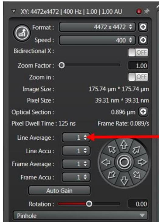
**Figure 3.15.** In order to decrease background noise, image lines and/or frames can be averaged. The number of times the image is scanned can be chosen via the dropdown menus. The dropdown menu for line averaging is indicated by the arrow above, but if it is desired to scan by frame, the frame average dropdown can be selected.
