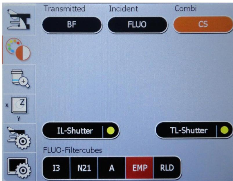
**Figure 1.11** Leica Smart Touch Panel Color Wheel icon overview. Under this icon, Brightfield (BF), Fluorescent (FLUO) or a combination of the two (CS) can be selected. The IL and TL shutters can be turned on and off by selecting the corresponding icon and various filters can be applied.
