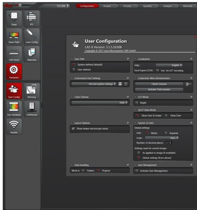
**Figure 2.10** LAS X Overview of the User Configuration Icon. Under this window, the last system settings and various system defined functions can be accessed. This icon is primarily used by the manager of the system.
