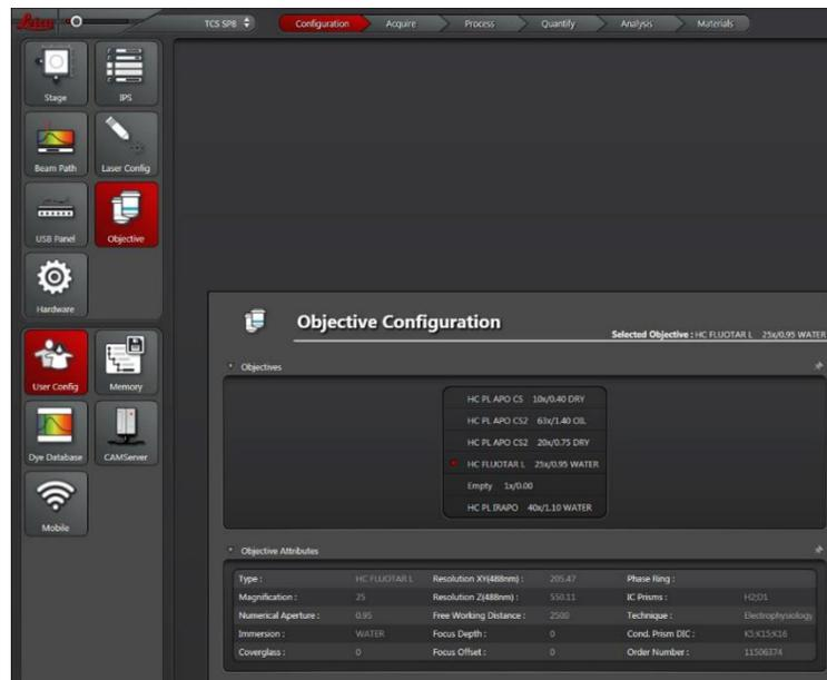
**Figure 2.8** LAS X Overview of the Objective Configuration icon. The objectives available are the 10X, 20X, 25X water, 40x oil, 63X oil, and a 25X Clarity objective that is installed on a need-be basis. In this figure the 25X Objective is selected and the corresponding specifications can be seen.
