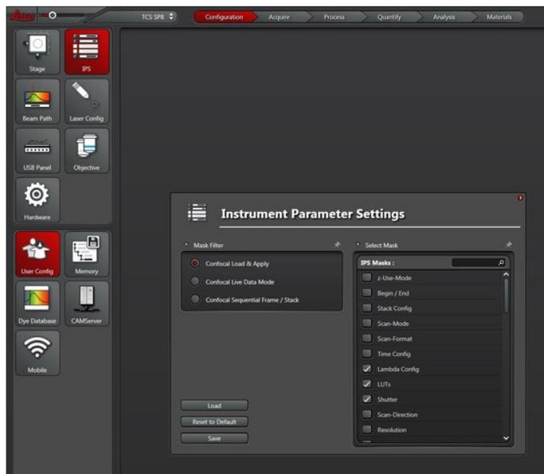
**Figure 2.4** LAS X Overview of the Instrument Parameter Settings. This screen provides access to specific software masks that are typically set upon instrument installation.
