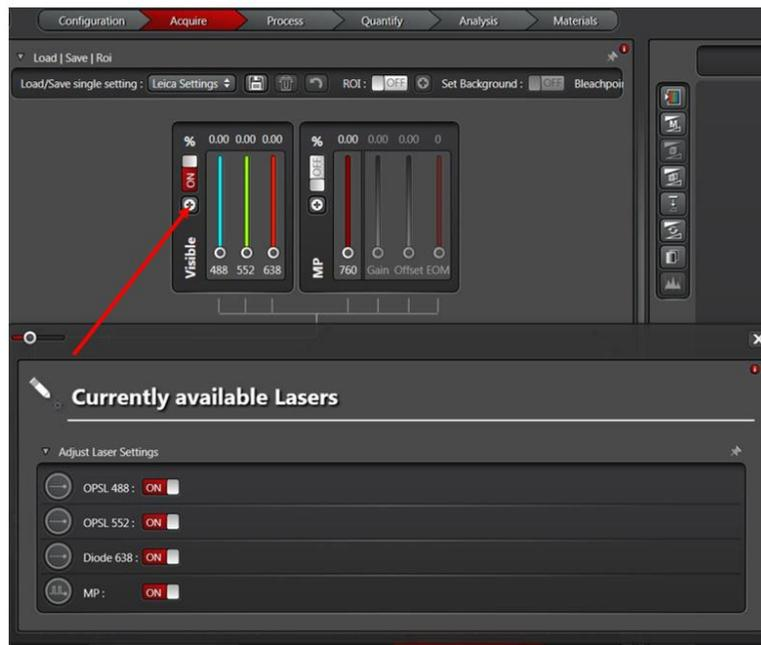
**Figure 1.7** Lasers can be turned on under the LAS X Acquire screen in the center panel (the Dye Database Panel). By selecting the “+” as indicated by the red arrow the currently available lasers can be seen and turned on. Only the lasers that will excite the fluorophore should be turned on as to preserve laser life of lasers not in use. There is redundancy in the system so it should be noted this is not the only screen the lasers can be turned on from.
