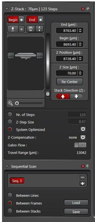
**Figure 3.17.** The Z-stack menu under the Acquire Window. For this specific Z-stack the beginning is set to 8693.40  $\mu\text{m}$  and the end is set to 8763.40  $\mu\text{m}$ . With the system optimization setting the optical slice is 70  $\mu\text{m}$ , with 123 steps, and each step size is 0.57  $\mu\text{m}$ . The Z-stack can be scanned between lines, frames (selected), or stacks as seen in the sequential scan box.
