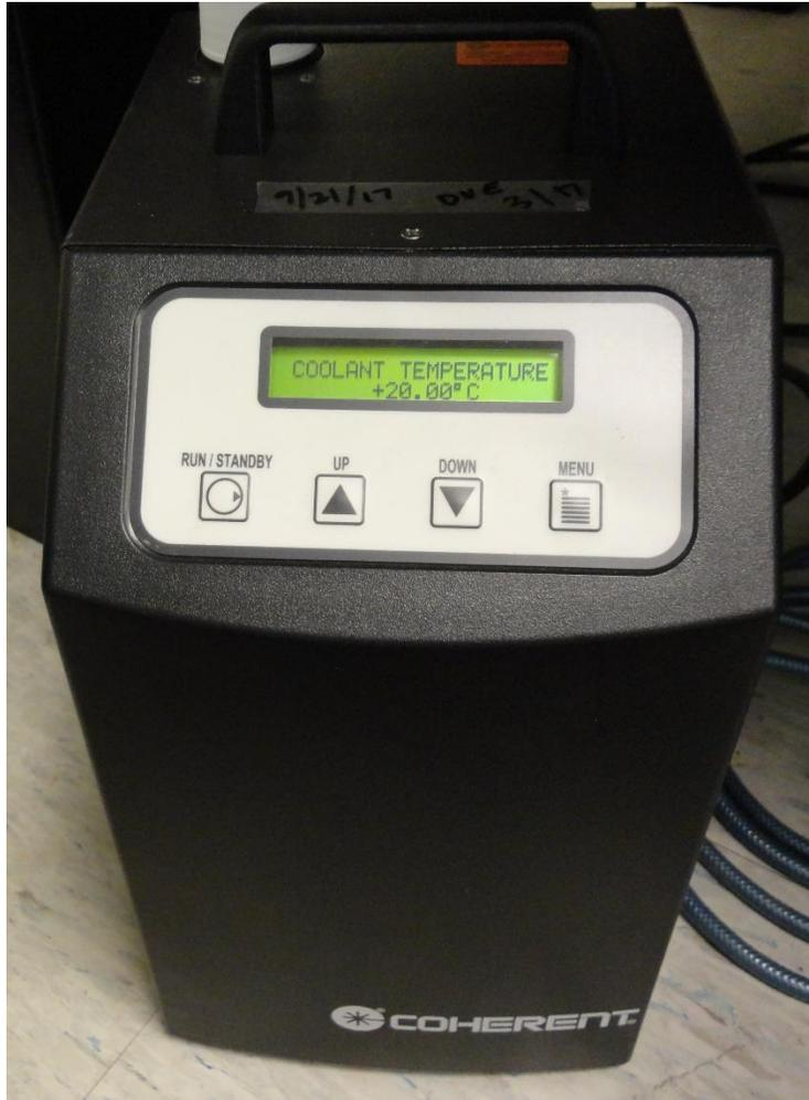
**Figure 1.2** Coolant should be verified and read no greater than 20.00° C before operation of the system.
