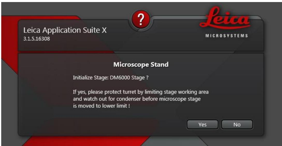
**Figure 1.5** Upon startup of the LAS X software, two pop up screens will prompt the user to set up various aspects of the Leica SP8 system. The second of these asks if the stage should be initialized. The stage only needs to be initialized if a tiling experiment will take place. Otherwise, “No” can be selected from this window.
