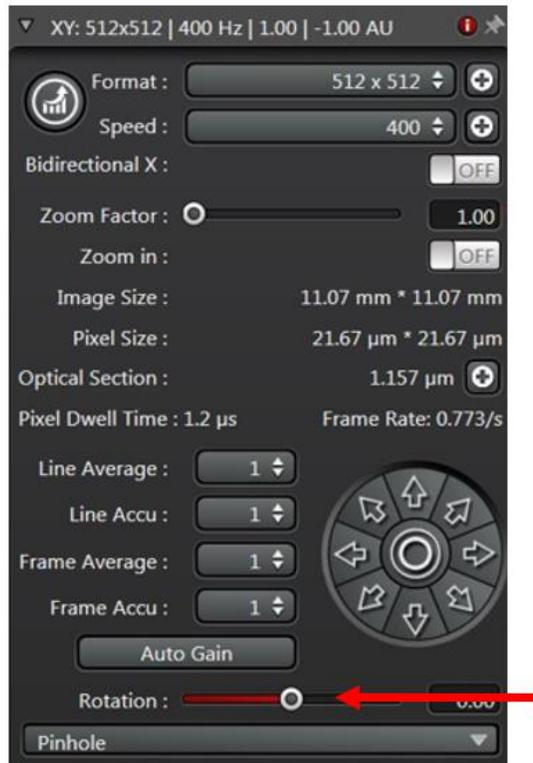
**Figure 3.11.** Images can be rotated, as indicated by the arrow above, within the LAS X software in order to identically align any desired images.
