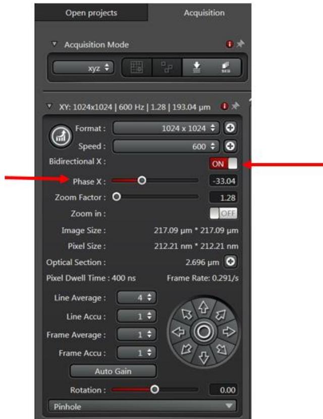
**Figure 3.8.** An image can be scanned in either a unidirectional (default) or bidirectional pattern. To turn on bidirectional scanning, the bidirectional button is selected as indicated by the right arrow above. Phase X (left arrow) compensates for any distortion created by bidirectional scanning.
