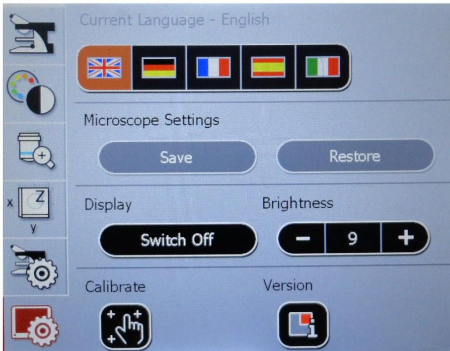
**Figure 1.15** Leica Smart Touch Panel System Setting icon overview. This icon will rarely, if ever, be used by anyone other than the manager of the system.
